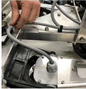
2. Repair any minor damage to the sheathing with tape.
