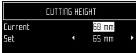
**Note:** If this value is negative, it implies that a reset of the parameters has taken place and that the blade height values need to be re-calibrated. See [The Service menu](#) (page 121).
