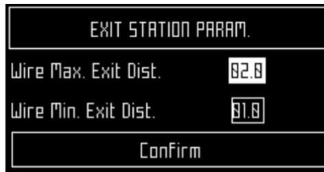
**Wire. Max. Exit Dist.** and **Wire. Min. Exit Dist.** are the minimum and maximum distances for which the robot will follow the wire (trackwire movement) when leaving the station. They are illustrated in the figure below.
