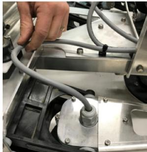
2. Repair any damage to the sheathing with tape.
