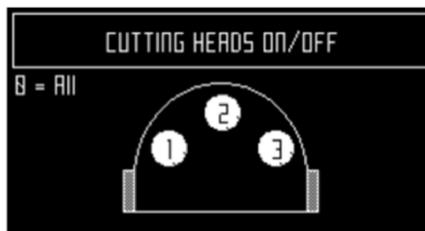
This figure indicates that all the cutting heads are enabled.
