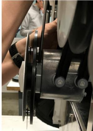
2. Undo the screw on the axle shown below.
