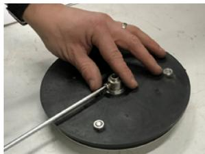
3. Undo the nut to remove the axle.
