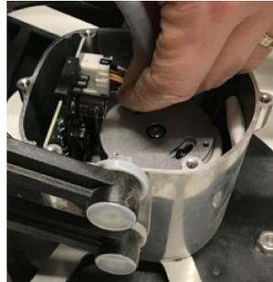
6. Visually inspect the interior of the motor. Check for dampness and dry it out if necessary.
