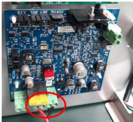
7. Take the cable behind the wire and positioning boards and push the other end into the socket on the positioning board.
