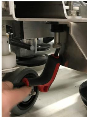
2. Place the new silentbloc in place in the position as shown below.
