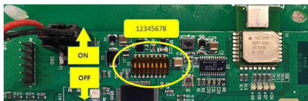
**Figure 39: Charging station type switches**
