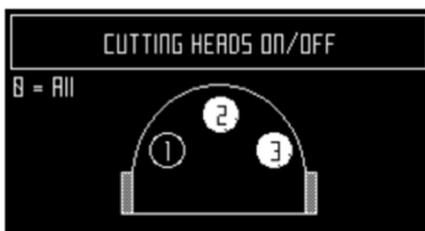
**Note:** Pressing **0** on the numeric keypad will select all the cutting heads.
