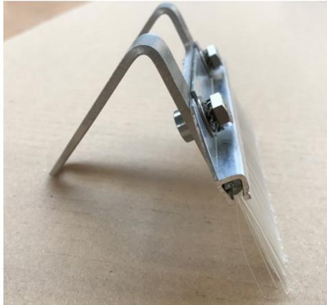
4. Screw the brushes onto the bracket, inserting the flat washer next to the brush and the crinkled washer below the screw head. Use a torque of 12Nm.
