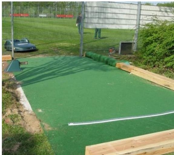
Figure 87: Charging station in narrow enclosure protected by the fence
