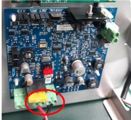
3. Connect the new cable to the wire board. Ensure the wire is properly screwed and secured.
